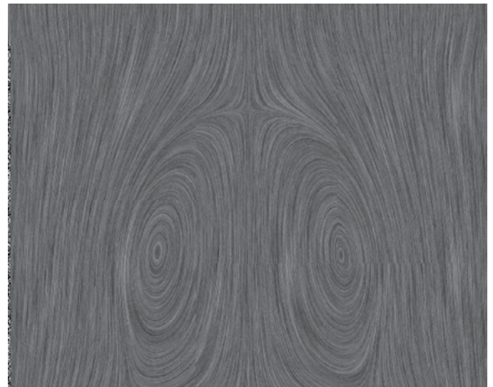
Figure 1: Line Integral Convolution from a vector field sampled over a uniform rectilinear grid
