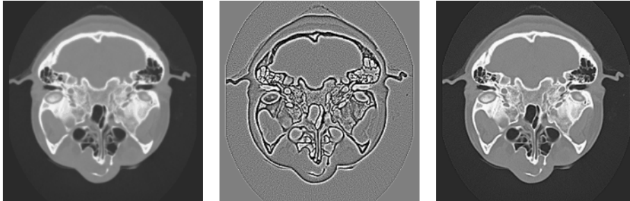
Figure 10-9 High-pass filters can extract and enhance edges in an image. Subtraction of the Laplacian (middle) from the original image (left) results in edge enhancement or a sharpening operation (right) ( EnhanceEdges.tcl ).
